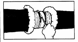
3. Pull jacket and insulation back over cores. Tape jackets together with at least 2 wraps of duct tape.
