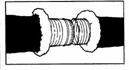
2. Tape cores together with at least 2 wraps of duct tape. Secure connection with 2 clamps placed over the taped core ends and past the beads.
