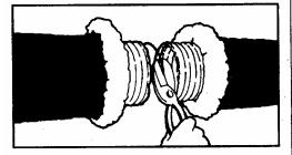
2. Slide at least 1<sup>e</sup> [25 mm] of core over fitting and past the bead. Seal core to collar with at least 2 wraps of duct tape. Secure connection with clamp placed over the core and tape and past the bead.
