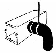
5. Vertically installed duct should be stabilized by support straps at a maximum of 6 feet (1829 mm) on center.
