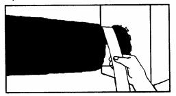
1. Fold back jacket and insulation from core. Butt two cores together on a 4" [100 mm] length metal sleeve.
