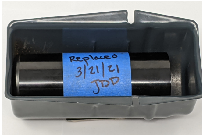
Figure 13. Label the replacement capacitor with a paint pen or tape and marker. This will allow easy identification if further problems occur with this motor.
