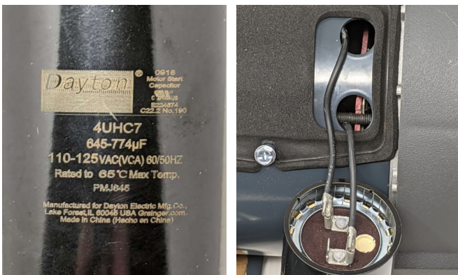
Figure 4. Start capacitor label information to be used in the evaluation worksheet (left). Photo to remember wiring arrangement and wire color (right)
