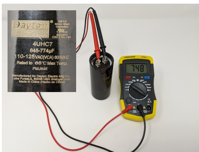
Figure 11. A capacitance meter is shown with the two probes placed on the two capacitor tabs. This capacitor label shows a capacitance of 645 to 774 \mu\text{F} . The meter is reading a capacitance of 748 \mu\text{F} , which is in the acceptable range. The capacitor is good.
