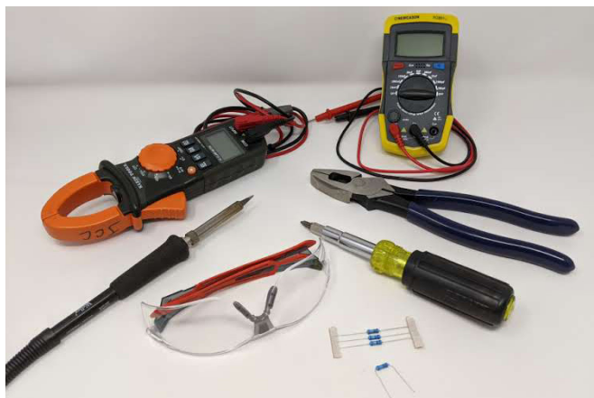
Figure 1. Tools to perform a motor capacitor test: electrical multimeter, capacitance meter (optional), insulated pliers, multi-tool driver, electrical resistors, and soldering iron. Always wear safety glasses.
