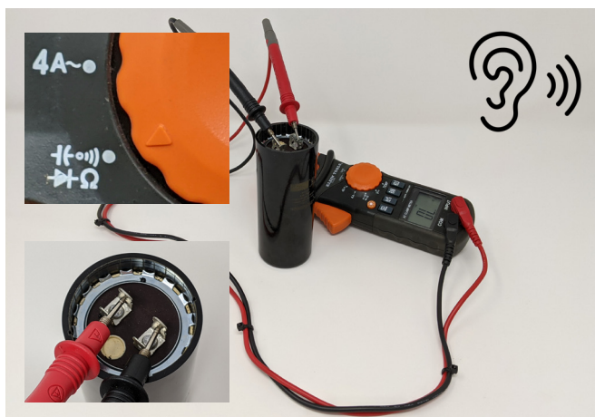
Figure 9. To test electrical continuity between the dielectric layers, turn the multimeter to the continuity position (upper insert) and then place one multimeter probe on each of the two tabs (lower insert). A beeping sound indicates that the capacitor is bad and should be replaced.
