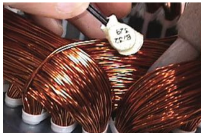
Figure 7.6 - Thermostat installation in the winding
