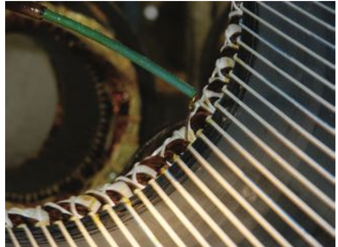
Figure 1.12.c - Resin applied by continuous flow process
