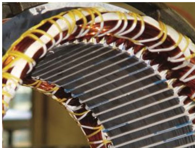
Figure 1.12a - Wires and films used on the stator
