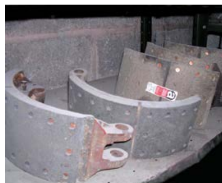
Figure 41 Asbestos brake linings for quarry vehicles
