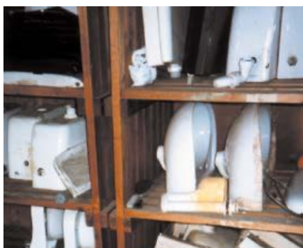
Figure 40 Asbestos-reinforced toilet cistern
