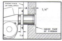
The Air Tube Length (Dimension A) is the distance from the front of the burner housing to the drain hole in the burner head. (NOTE: Adjustable flange width - 7/8'').
