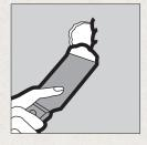
c. Crisscross two or three strips of joint tape over opening and embed tape in joint compound. Let harden.
