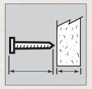
Drive nails in straight, not at an angle. Do not overdrive or countersink nails. This results in breaking the face paper or fracturing the gypsum core. If a nail happens to go in crooked, hold the panel tight against the framing and drive a second nail in about 2" from the nail that punctured the paper. Then drive the first nail in below the surface of the board.
