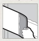
Apply pressure to knife edge farthest from the joint and lift the other edge just slightly above surface. Draw knife down joint. Repeat for opposite edge. This technique is called feathering. Joint compound should extend beyond first coat for a total width of 7" or 8".
