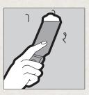
b. To repair a small hole or crack, trim any loose pieces from the damaged area and wipe it clean. Fill with joint compound, using a putty knife. Let harden. Add second coat if necessary. Sand and prime when dry.
