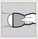
Then raise the knife blade to a more upright position and scrape off excess with a second stroke at a right angle to the first stroke. Compound should be level with panel surface.
