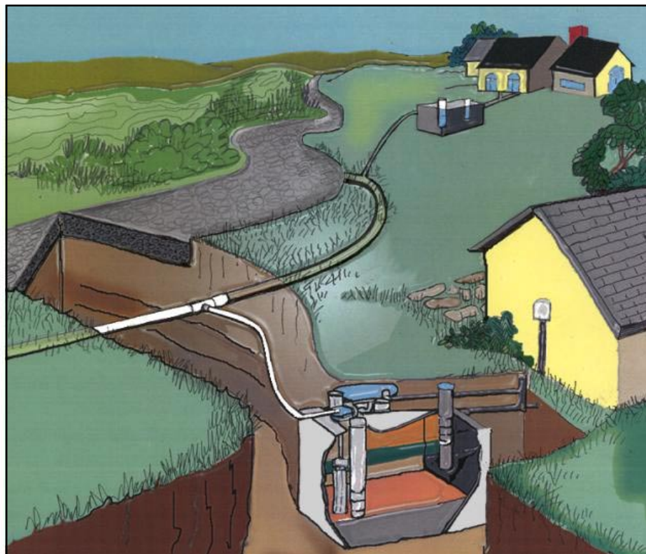
STEP systems use septic tanks to remove larger solids and small pumps to transport the sewage effluent.
