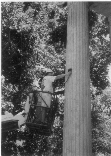
Fig. 11. Impulse radar is being used to evaluate both the orientation and depth of cracks visible on the surface of the column shaft. Photo: Edmund P. Meade, P.E.
