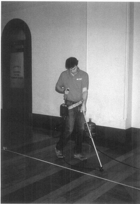
Figure 2. (a) The floor structure is scanned using impulse radar. An operator is shown, pushing the transducer across the floor surface at a constant speed. (b) The transducer is being pulled, by machine, at a constant speed. Photos: Marie Ennis, P.E.
