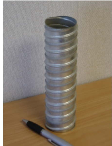
Drossbach tubes are embedded vertically in the bottom edge of the Litecrete panels
